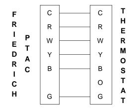
NOTE: B terminal used on heat pump models only
